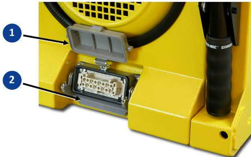
Fig. 9-5 Remote starting device with HARTING® socket
