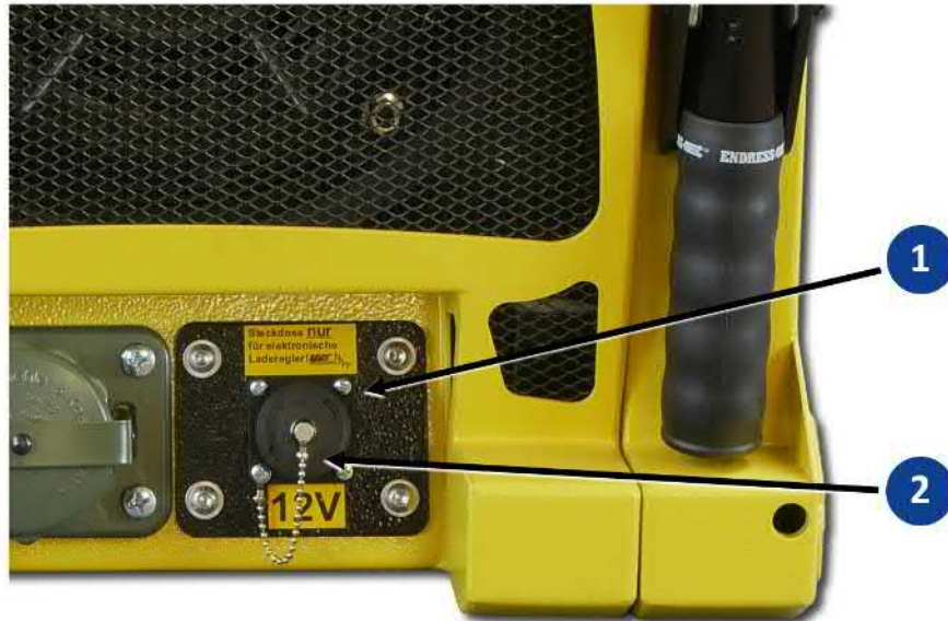
Fig. 9-2 BEOS charging current socket
