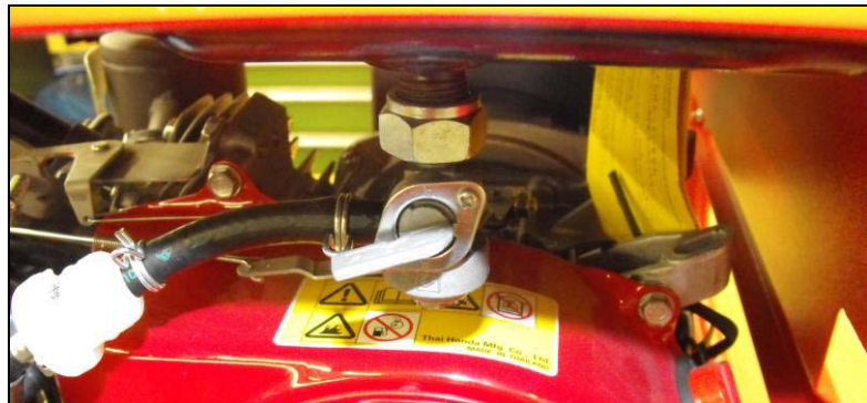
Fig. 4.5: Close the fuel valve
