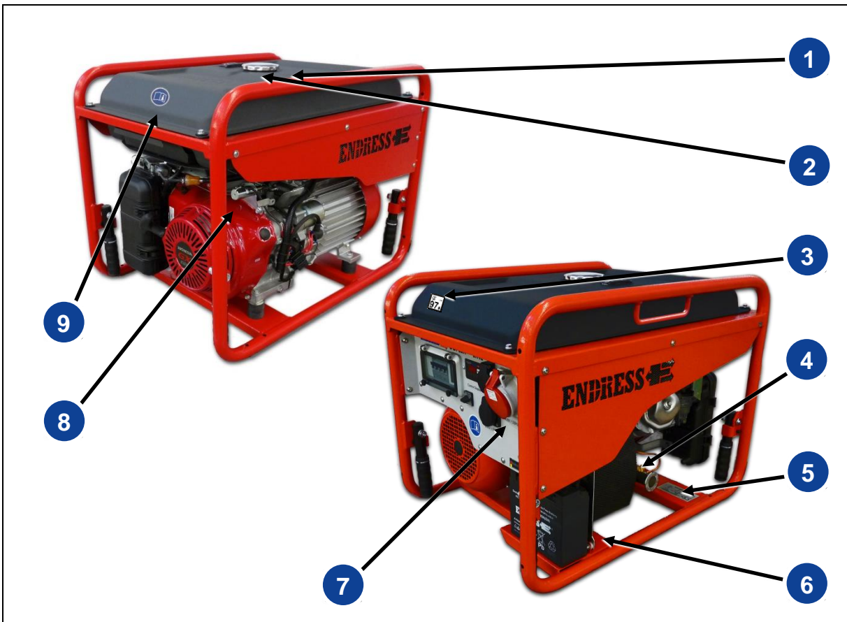
Figure 2-1: Signs on the generator
